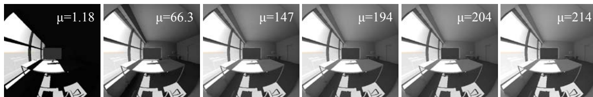
Figure 2 RPICT renderings with number of ambient bounces ranging from 0 (left) to 5 (right). Adding ambient bounces increases the overall radiance of the scene originating from the sky, though the effect is imperceptible beyond five bounces. Mean image luminance ( \mu ) is shown in \text{cd}/\text{m}^2 .
