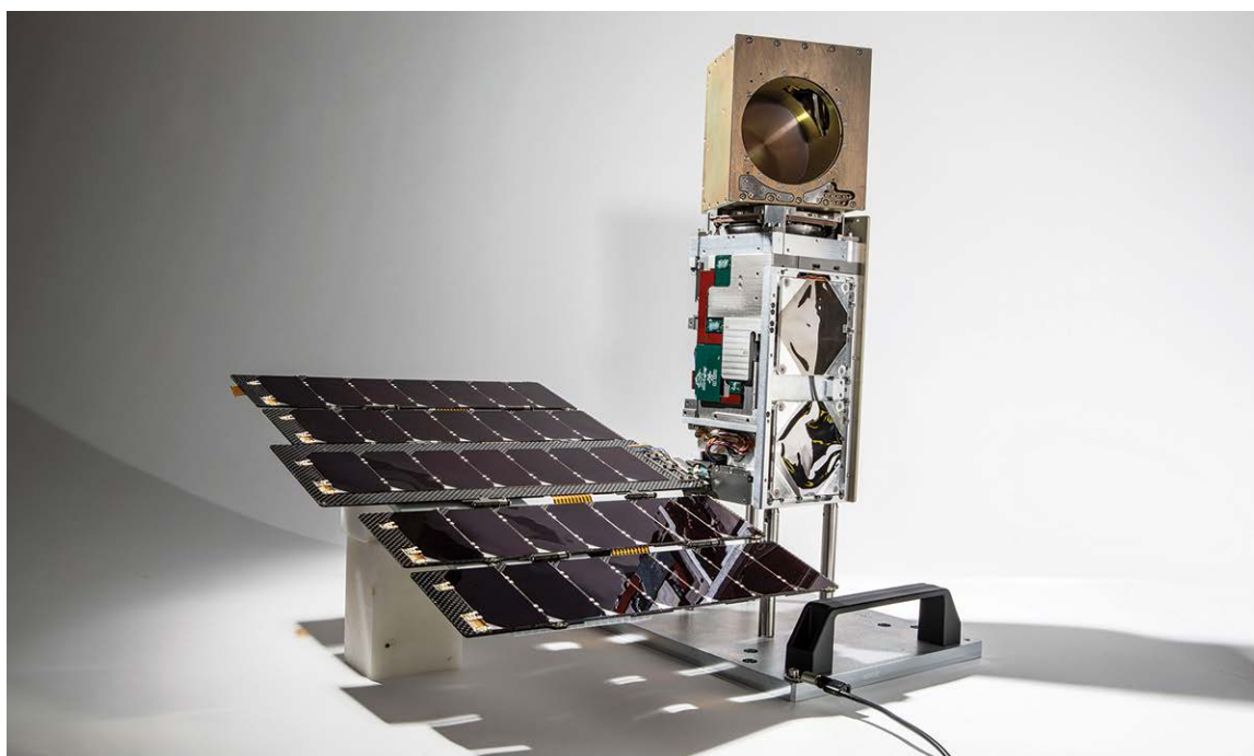
Figure 2. The TROPICS CubeSat is shown with its solar array deployed. All six of the CubeSats have successfully completed space vehicle environmental testing.
