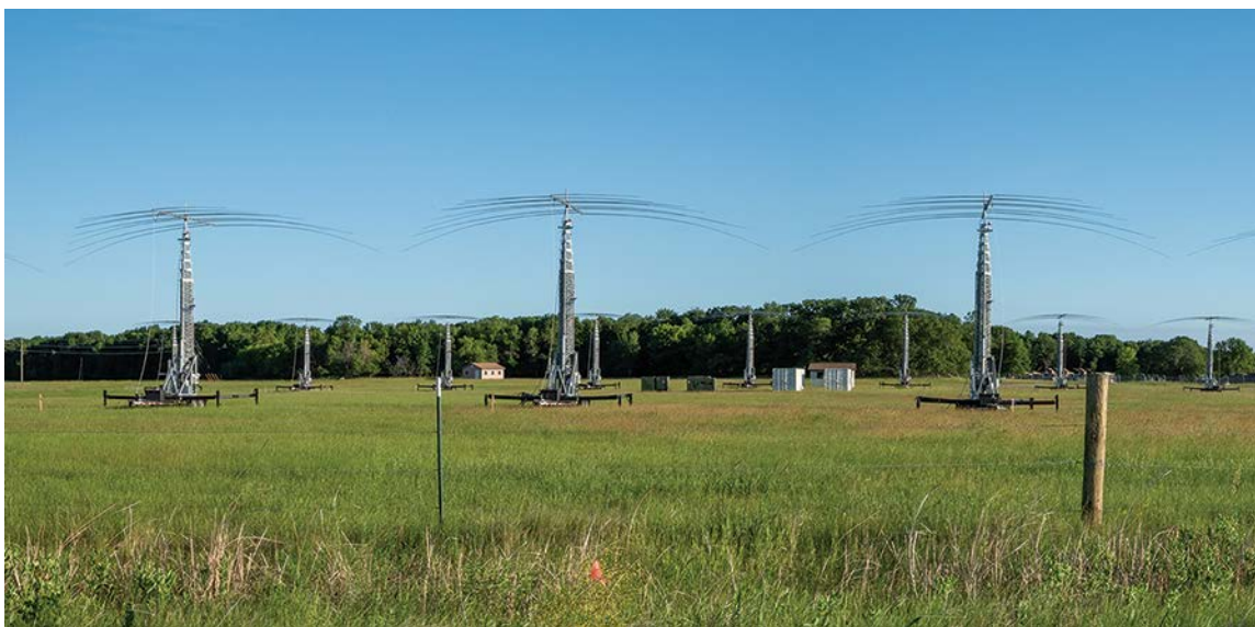
Figure 3. Over-the-horizon radar (OTHR) can potentially support long-range surveillance of the polar region but is hindered by interference induced by the Aurora Borealis. To study the performance of clutter mitigation algorithms, the laboratory designed, developed, and deployed a full-scale OTHR to North Dakota.
