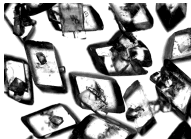
Figure 15. Microscopy image of paracetamol product crystals obtained from run 2 (250 \times ).
