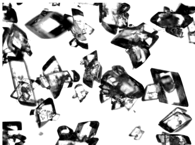
Figure 13. Microscopy image of paracetamol product crystals obtained from run 1 (250 \times ).
