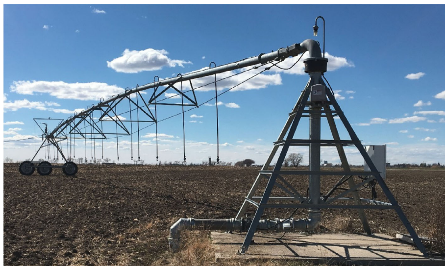
FIGURE 8 A 1-segment central pivot. The length of the arm is 50 m. A typical central pivot usually has a few segments with the total arm length about 300 to 400 m [Color figure can be viewed at wileyonlinelibrary.com ]
