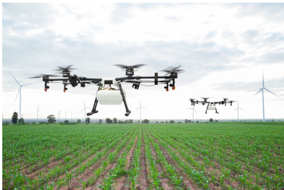
FIGURE 10 Agriculture drones with centimeters per pixel resolution cameras can be trained to detect changes in leaf color to infer water and nutrient needs of crops. Computer vision methods can be developed to detect and identify different weed types [Color figure can be viewed at wileyonlinelibrary.com ]
