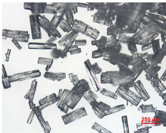
Figure 2. D-Mannitol crystals after the conditioning process with uniform shape and size.
