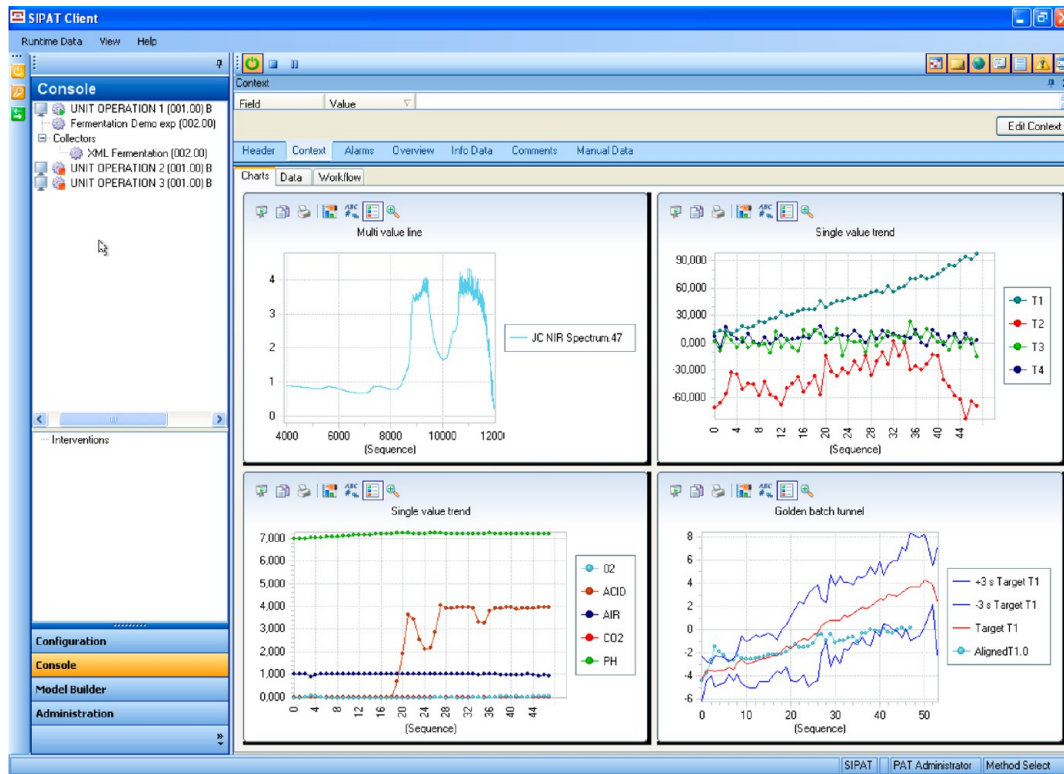
Figure 67. Runtime screen from a PAT application, including spectral NIR data (upper left), process data (lower left), calculated parameters (upper right), and a golden batch trajectory (lower right).
