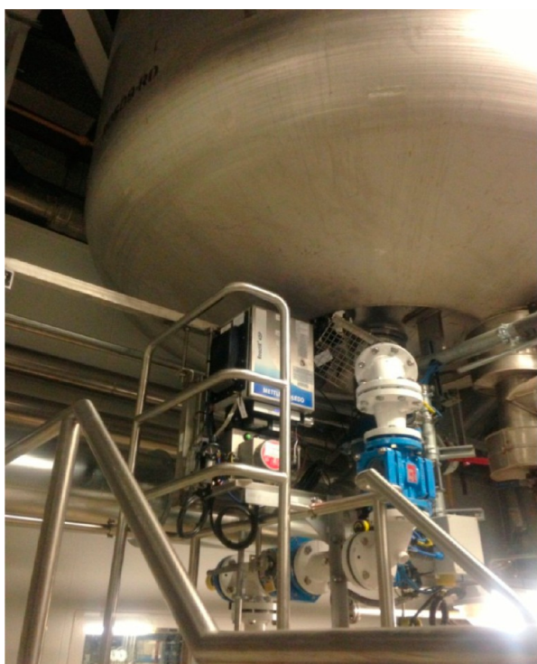
Figure 65. Installation of the Mettler Toledo 45P mid-IR at the bottom of the tosylfuranoside reduction reactor.
