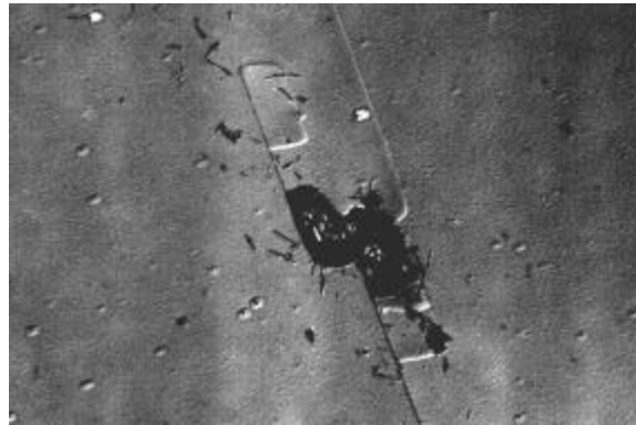
Figure 5.10 Nomarski interference contrast image (200x magnification) of the surface of the structure depicted in Figure 5.2. The slip lines and wire-like pieces are the result of oxidation of the AlAs layers in the DBR. Any visible vertical and horizontal striations are caused by the printer.
