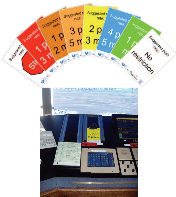
Fig. 2: (Top) Color-coded cards that were used to communicate the suggested pushback rates. (Bottom) Display of the color-coded card in the Boston Gate Controller’s position.
