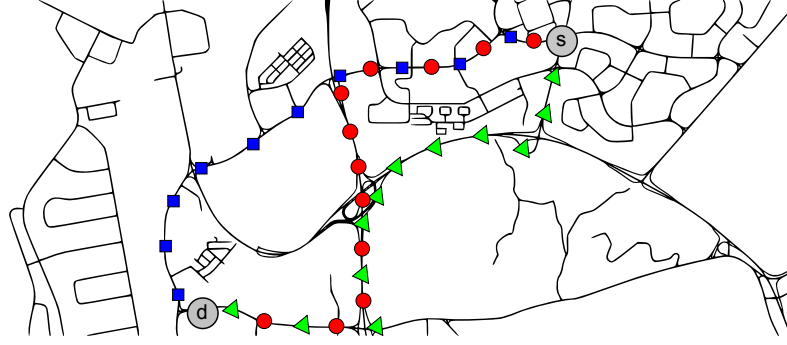
Figure 4 Local map. s and d locate the departure and arrival nodes. Three paths are highlighted. The left one (blue) is 5.3-km long and takes 9 minutes to travel. The middle one (red) is 6.4-km long and takes 8 minutes to travel. The rightmost one (green) is 6.1-km long and takes 10 minutes to travel.
