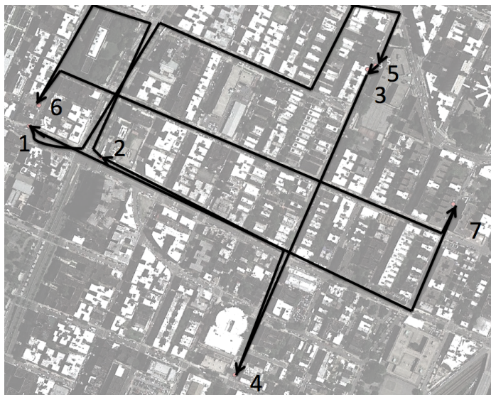
Figure 12: Sequential formulation route: 1-5-3-4-2-6-7-1. The simultaneous formulation also chooses this route when C_1 is small.
